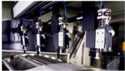
Multiple laser heads perforate plastic and paper in-line
